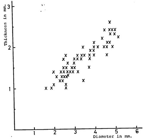
Fig. 2. Scatter diagram showing the relation between the diameter and thickness of the megalospheric tests.
