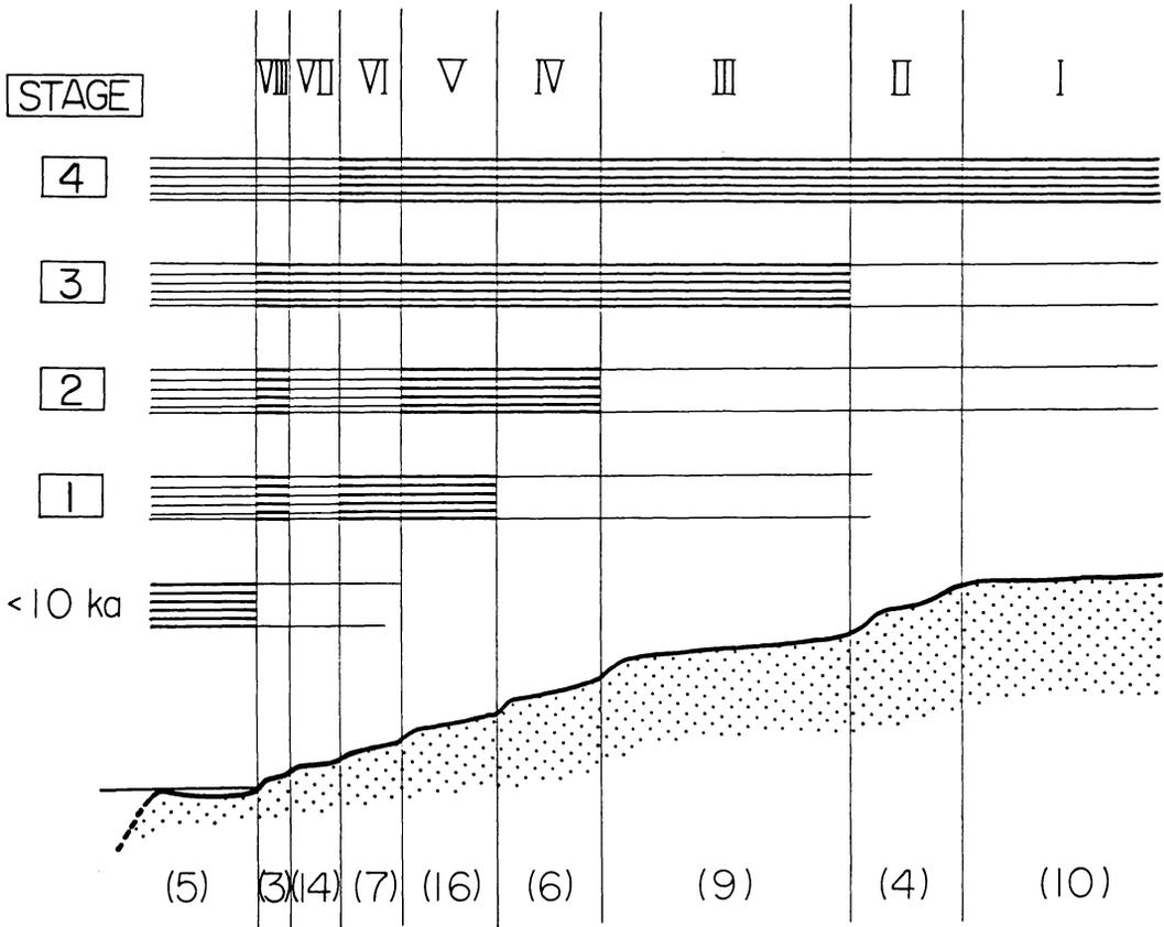
Text-fig. 2. Schematic illustration of eight steps of marine terraces on Hateruma. (Topographic cross-section is drawn not to scale. Roman numerals indicate the morphostratigraphic units of Ota *et al.*, 1982. Parenthesized figures mean number of coral samples dated. See text for details.)
