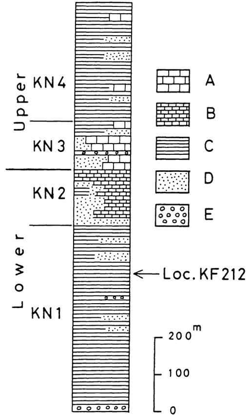
Figure 2. Columnar section of the Kanokura Formation of the Kamiyassee district, showing the stratigraphic position of the fossil locality (KF212). A: massive limestone; B: bedded impure limestone; C: shale; D: sandstone; E: conglomerate. (Redrawn, and adapted from Tazawa, 1973).
