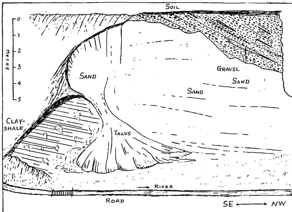
Text-Figure The Kayama clay-shale exposed by weathering.
