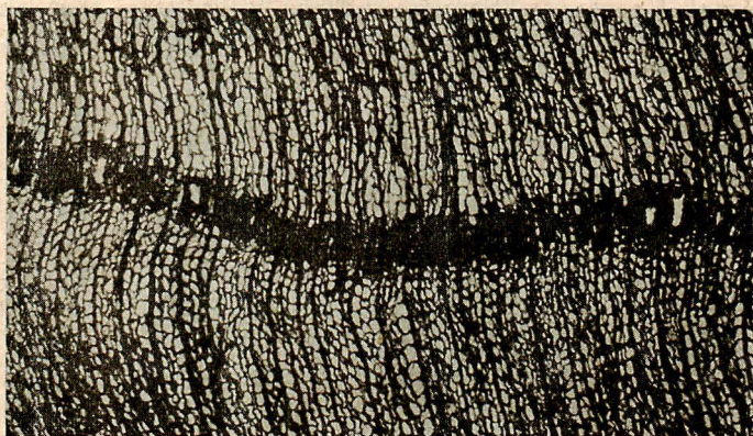
Fig. 4. Transverse section of the Wood, showing traumatic resin canals.
