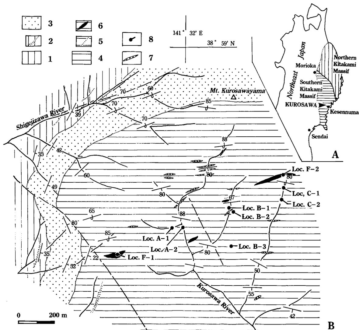
**Figure 1.** Index map (A) and geologic map of the Kurosawa district, northern Kesennuma, Southern Kitakami Massif, Northeast Japan (B). 1-2. lower part of the Ochiai Formation (1: shale, 2: sandstone). 3. Toyazawa Member of the Ochiai Formation (sandstone, limestone, shale and conglomerate). 4-6. middle part of the Ochiai Formation (4: shale, 5: thin sandstone, 6: limestone). 7. porphyrite. 8. fossil localities.
