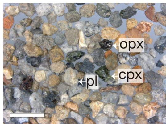
Figure 3. Pictures of the sediment from size fractions 0.5–1, 1–2 and 2–4 mm for stations N9 (left) and N12 (right). Mineral abbreviations: pl: plagioclase; ol: olivine; cpx: clinopyroxene; opx: orthopyroxene. Bars = 1 mm.
